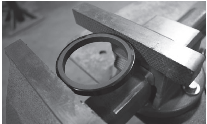
Figure 22 Model 361 Piston Ring Vise Break Method (Step 2)
