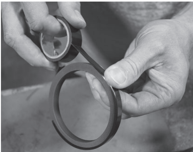
Figure 21 Model 361 Piston Ring Vise Break Method (Step 1)
