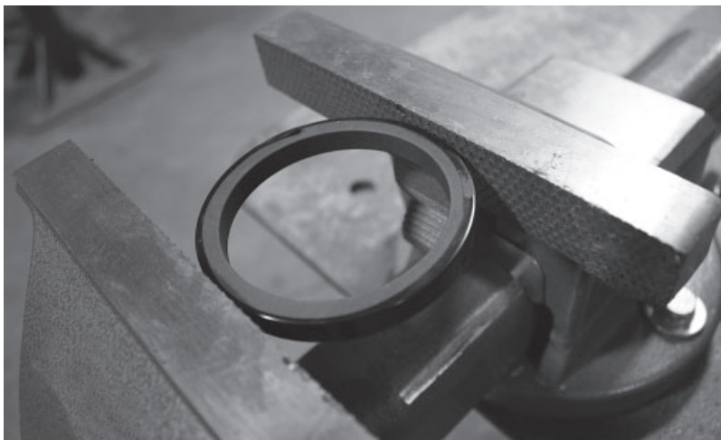
Figure 21 Piston Ring Assembly for Model 391 Valves (Step 2)
