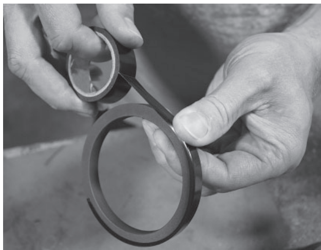
Figure 20 Piston Ring Assembly for Model 391 Valves (Step 1)
